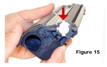
10) Remove the doctor blade cover by prying up the three tabs as indicated. Remove the cover. See **Fig. 16**
