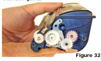
26) Install the black reset assembly so that the gears mesh, and the u-shaped section of the assembly is against the round post. If the assembly is set further out, the printer will not be reset. See **Fig. 33**
